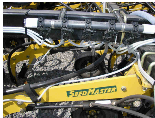
A seeding machine with VeriFlow2
