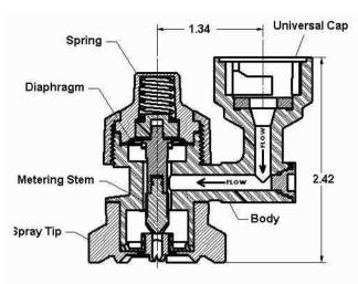
Hi-VariTarget is a nozzle that is capable of controlling flow rate and maintaining proper spray pattern and droplet size over an extended range of flow rates. The nozzle comprises a flexible spray tip that is automatically and appropriately deformed by a flexible metering assembly in response to changes in liquid pressure.
